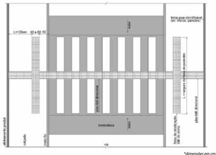
Figura 32 – Travessia com lombotaxa
